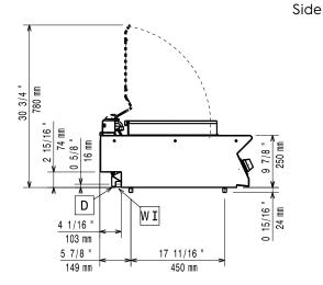
Drain Electrical inlet (power) ΕI
